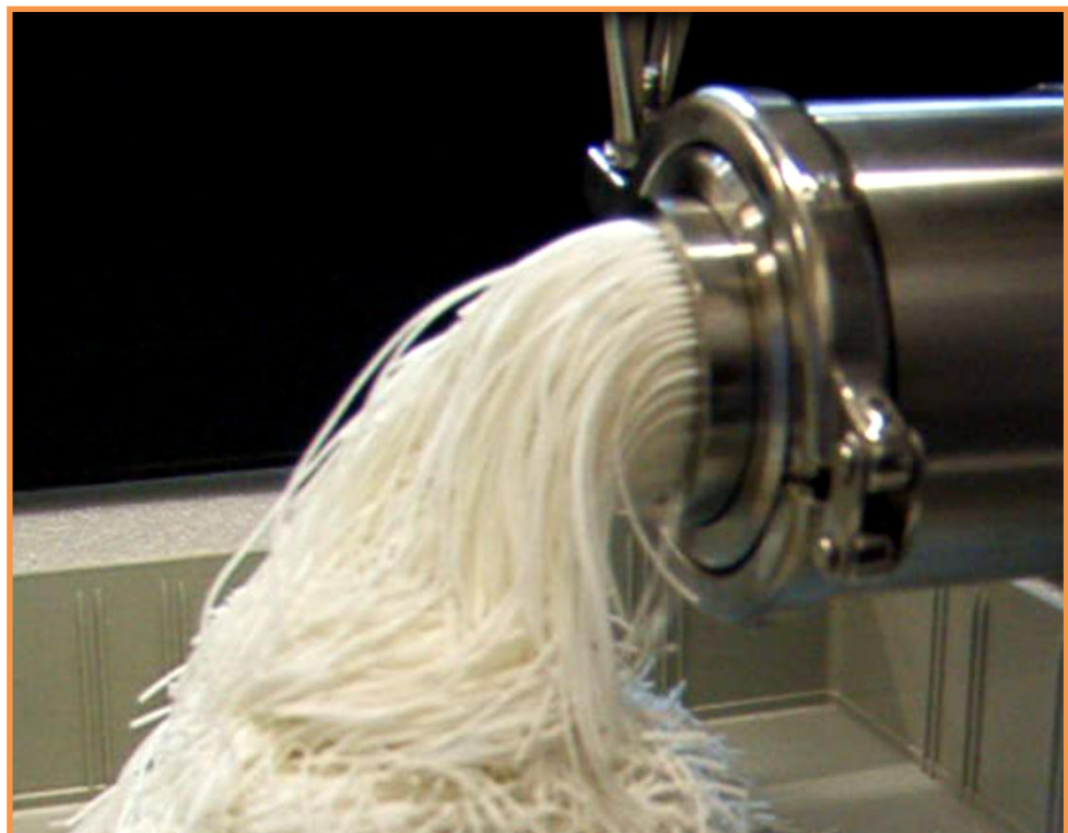
Axial Extrusion through 1mm wide and 4mm deep extrusion holes
