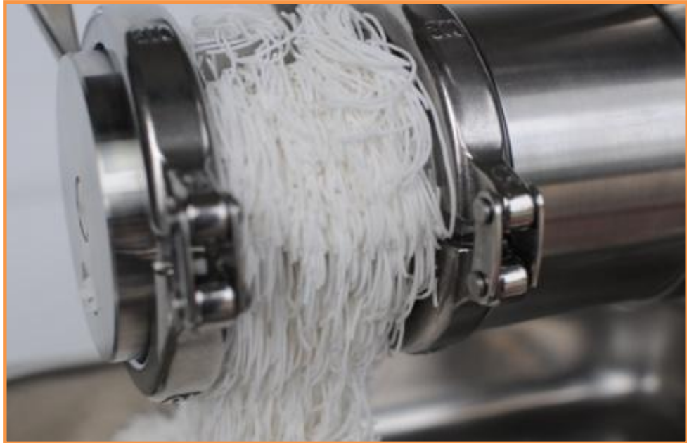
Axial Extrusion through 1mm wide and 4mm deep extrusion holes
